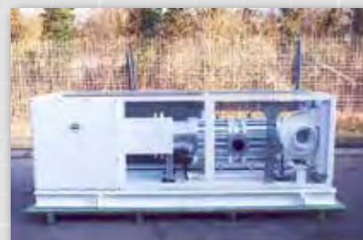
Brown Coal Gas Degasification Inlet 225°C (437°F); Design 280°C (536°F)
