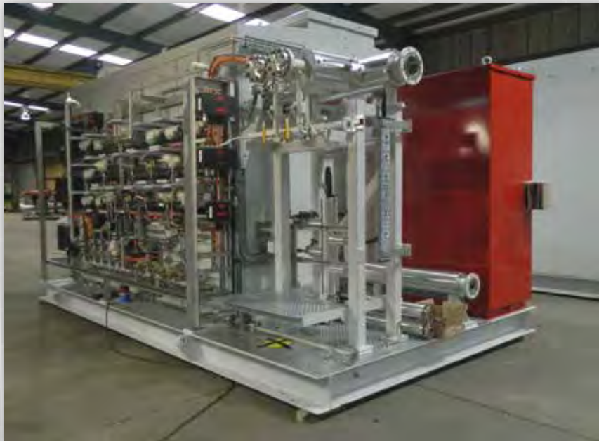
H 2 S Acid-gas Blower Package with Fire-suppression System
