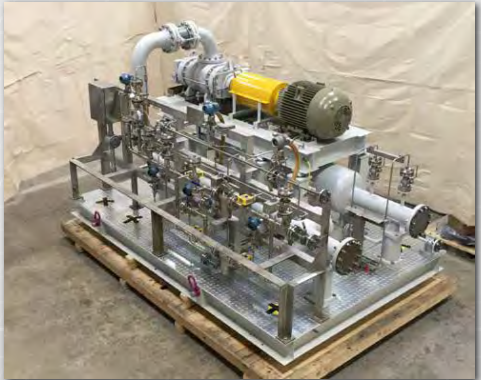
Regeneration Blower Package
