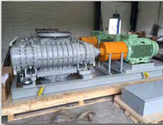
Vapor Recovery Vacuum Booster
