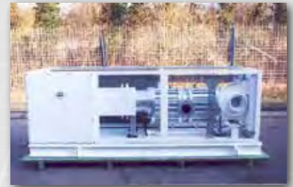
Brown Coal Gas Degasification Inlet 437°F (225°C); Design 536°F (280°C)
