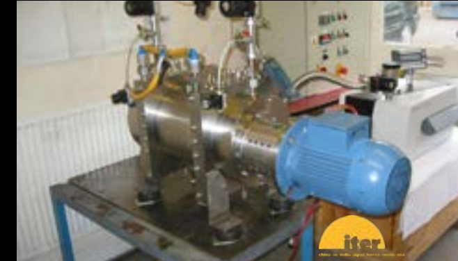
TRITIUM VACUUM CIRCULATOR (Nuclear Fusion Prototype - Attested by ITER for leak rate of 10^{-8} mbarL/s)
