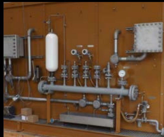
Seal Oil Supply System to API Standard 682, Plan 53B
