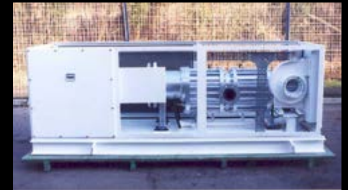
BROWN COAL GAS DEGASIFICATION Inlet 437°F (225°C); Design 536°F (280°C)
