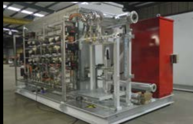
H 2 S Acid-gas Blower Package with Fire-suppression System
